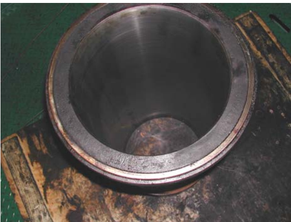
Fig. 11: Cylinder liner after cleaning
