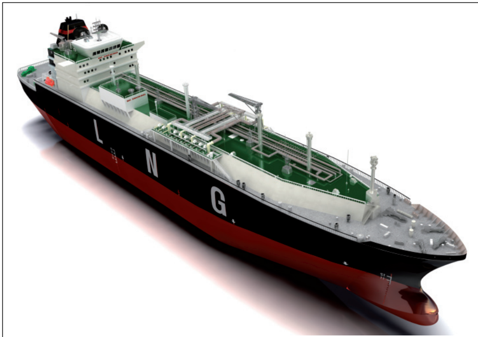
Fig. 4: Largest LNG carrier with DFDE propulsion (5 x 8L51/60DF) ordered by Spanish owner EN Elcano at Korean yard STX Shipbuilding
