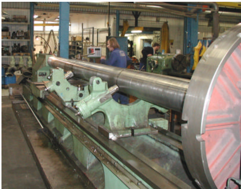
Final grinding of the shaft's coupling flange end
