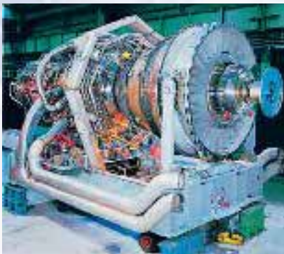
4 FT8 Gas Generator
