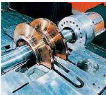
5 Inner bundle of RV090 Compressor
