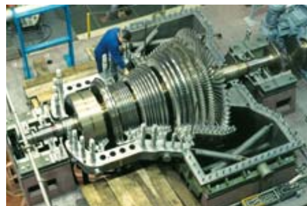
Fig. 15: Condensing Steam Turbine on Test Field
