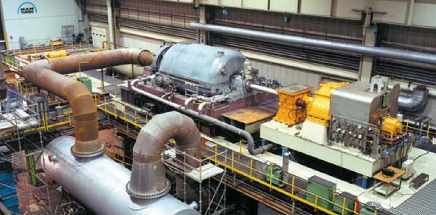
Fig. 12: Test Arrangement of Axial Flow Compressor
