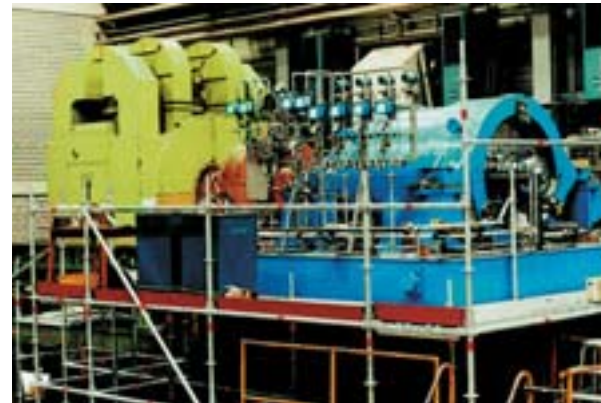
Fig. 14: Nitrogen HP Compressor on Test Field
