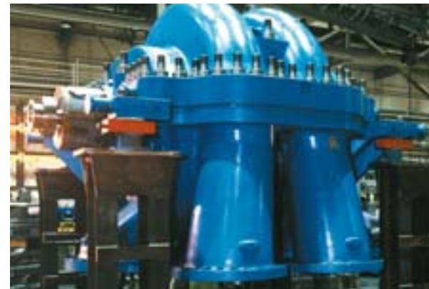
Fig. 13: Nitrogen LP Compressor
