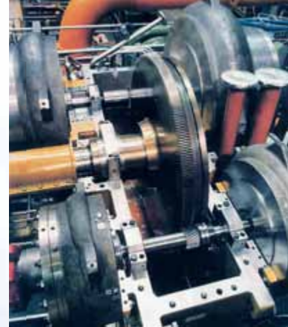
4 Bull gear with double modulus
