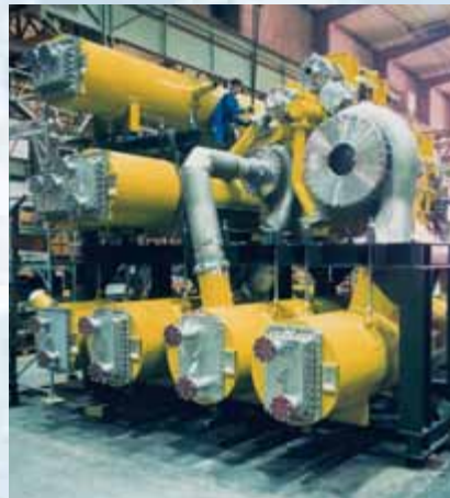
6 Compressor with complete cooling system in the assembling bay at our Berlin works
