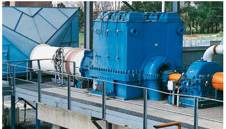
Air compressor RIK 100 in an air separation plant
