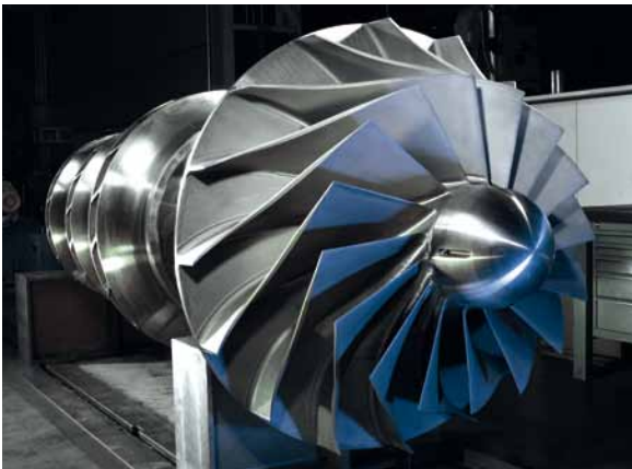
Latest development RIKT: First stage with axial inlet designed as open, overhung-mounted impeller
