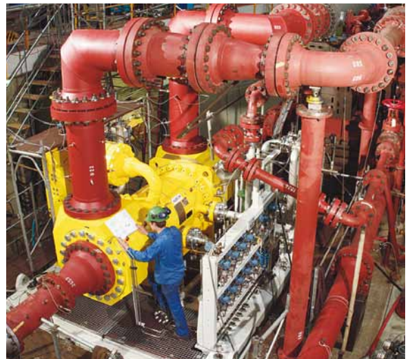
Works test of a MOPICO® unit
