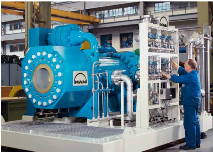
Fully assembled pipeline package
