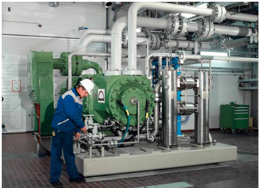
5 The tandem HOFIM™, both conventional and Sealed versions, offers the added capability of operating the two casings either in the series or in the parallel modes. This allows the operator to cover the widest possible duty range at highest efficiencies. Switching from one mode to the other can be effected during operation without shutdown.
