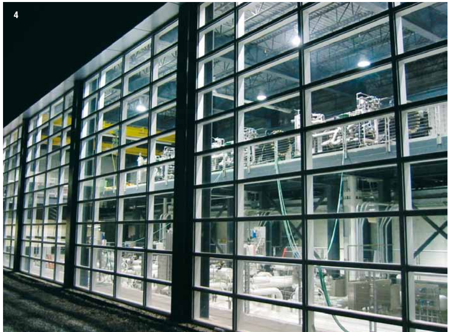
4 The first three HOFIM™ Sealed units operating in a gas storage facility in the USA. The plant layout allows the three units to operate in parallel, but also two units in parallel, feeding the third unit in series for high-pressure ratio requirements. Each motor is rated at approximately 7 MW. Gas can be compressed from 55 up to maximum 220 bar.
