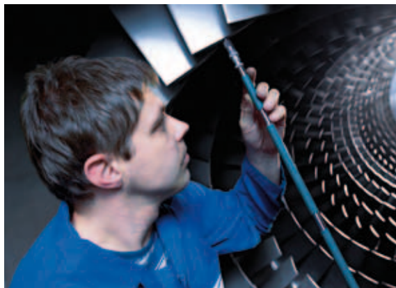
Final check of the new stator blade carrier
