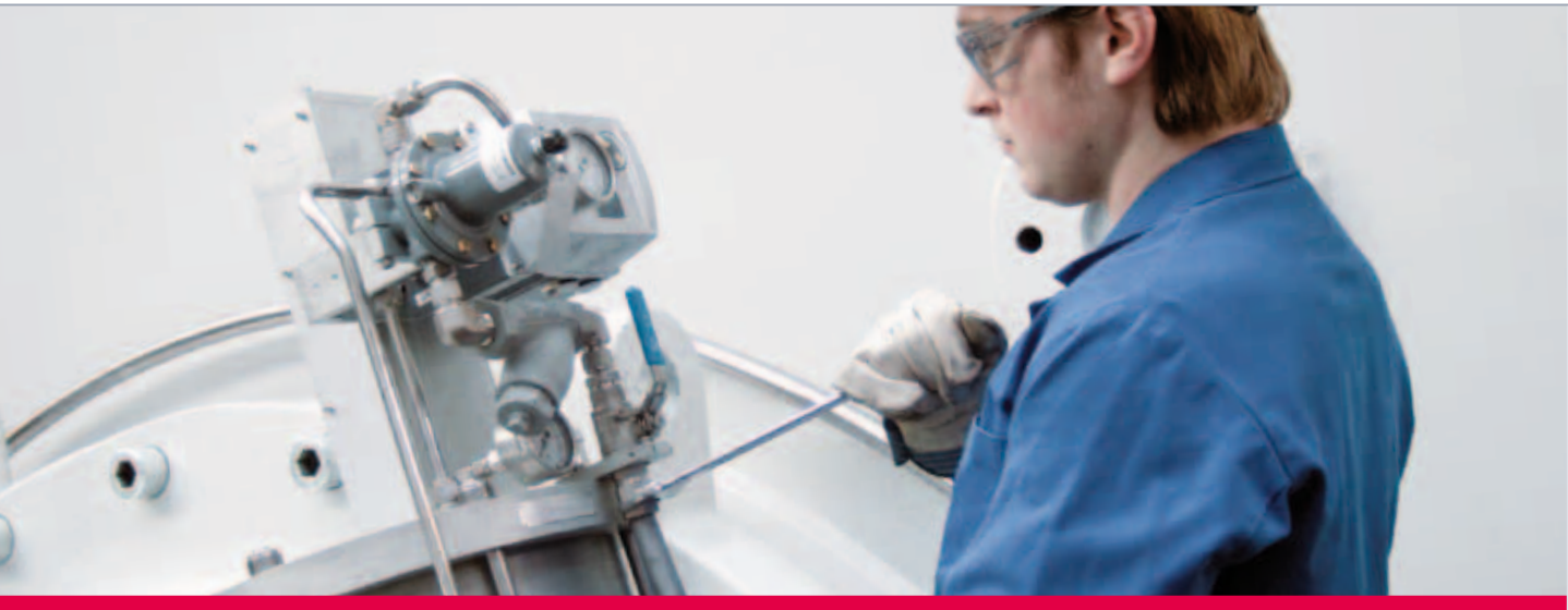
Assembly of guide vane actuating unit
