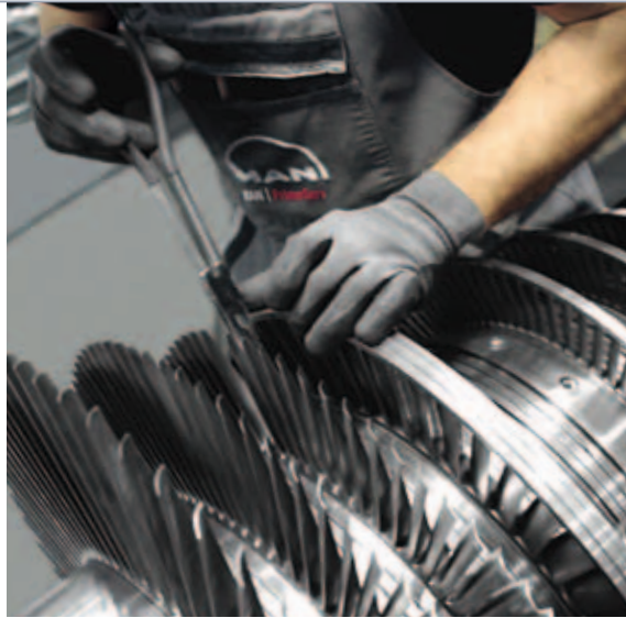
A service specialist applies a specifically made tool to adjust the sealing strips between the rotor blades on a turbine rotor.
