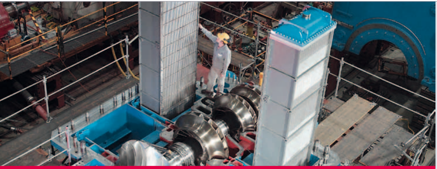
Assembly of plate fin coolers into an isotherm compressor
