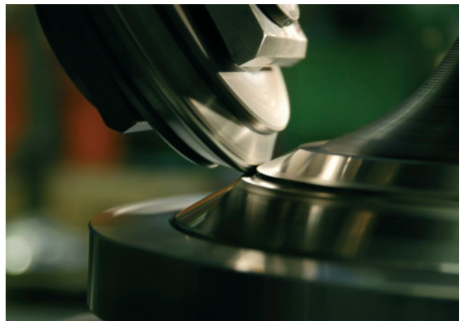
High pressure rolling on the welded spindle seat
