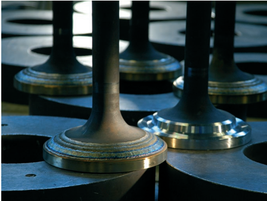
The spindle on the right shows the seat before the welding process
