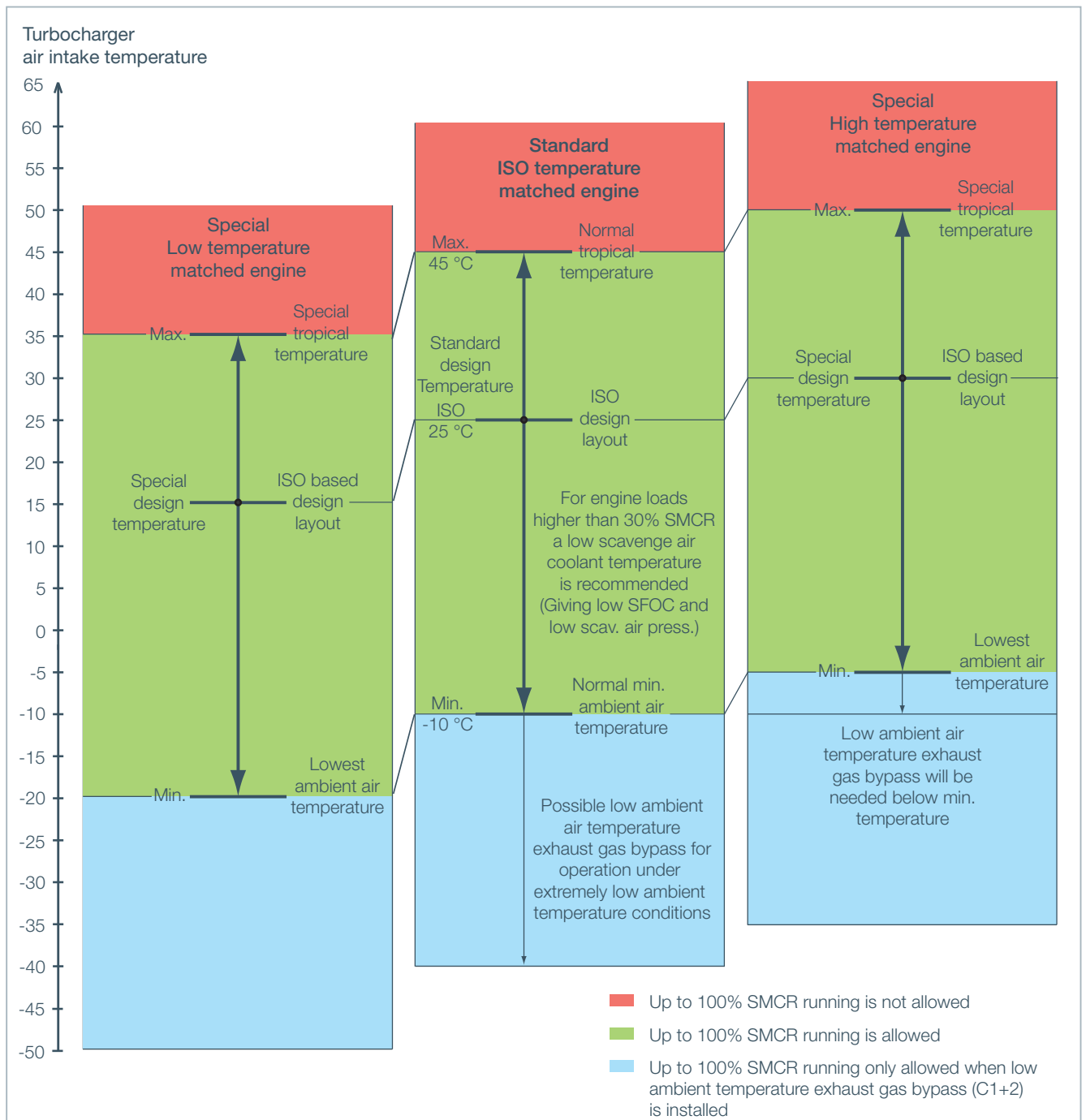
Fig. 2: Principles for standard and special high (or low) ambient air temperature matched engines
